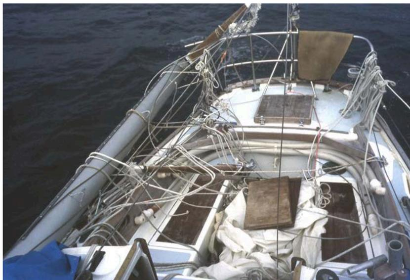
By using a sheet winch, I manage to bring the mast to a horizontal position, and then, with the help of tackles, I hoist it to deck level. Now that the halyards are no longer slapping against the rail from the constant rolling of the sea, I feel a great sense of relief.
