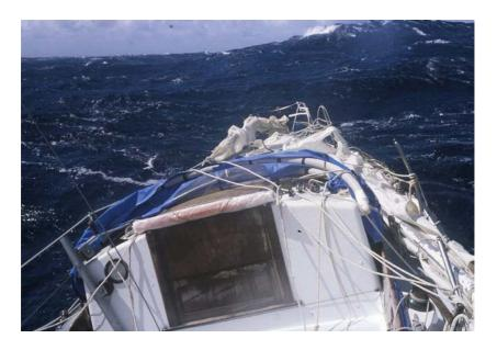
from chafing on the ragged edge of the mast. At least I manage to limit the damage to the rail from the repeated slamming of the shrouds and to lash the other section along the side deck.
