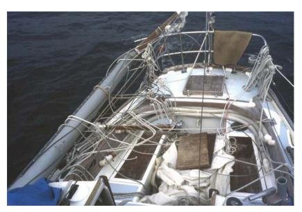
By using a sheet winch, I manage to bring the mast to a horizontal position, and then, with the help of tackles, I hoist it to deck level. Now that the halyards are no longer slapping against the rail from the constant rolling of the sea, I feel a great sense of relief.
