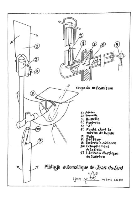
The system I invented solves this problem with a single piece of bent stainless steel quarter-inch rod: first two  $90^{\circ}$  elbows form a crank (4) that transforms the movement of the rod from vertical to rotary, then in the form of a horizontal "Z" (5). The central branch of the "Z" goes through a slot (6) cut through the stock of the servopendulum blade.
