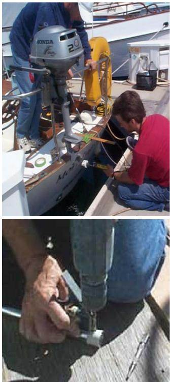
The struts are cut to the appropriate length, (the tube has one turnbuckle-type end, which allows for 2 inch adjustment of its length) and a ¼ in. hole is drilled through it, ½ in. from the end (make sure this hole is drilled at 90°) for bolting to the flat U-shaped bracket which will be bolted under the deck or to the hull, whichever is more convenient.
