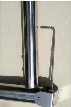
At the end of the autopilot ram, there is a hole made for connecting a vertical pin on the tiller. Turn the ram  $\frac{1}{4}$  turn, drill this hole all the way through with a  $\frac{1}{4}$  in. drill, and insert the L-shaped rod through this hole. Insert the dovetail-shaped plastic connector at the other end of this rod into the corresponding piece, at the end of the horizontal control axle.
