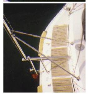
Provided some angulation between them is kept, **the braces do not need to be placed symmetrically**. One of them can be placed almost fore-and-aft, and the other to one side, **to allow passage** through the stern on one side.
