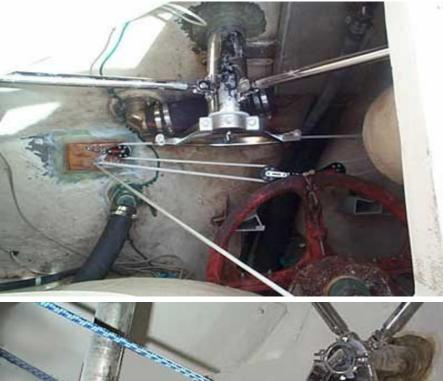
**CH** quadrant mounted down. Lines led to blocks fastened to pads bonded to the hull. Lines look like they are crossed, but actually, they are not : they pull directly from the other side of the steering quadrant. (Union 36).
