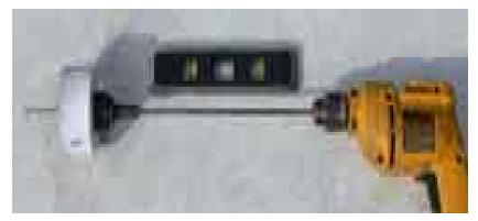
The secret is to maintain the tool very steady, level and parallel to the centre line; this way, you will easily cut through the transom, even if it is at an angle. Or through the curved surface of a canoe stern. If the drill is held very steadily, the hole-saw will not bind. If possible, cut half the thickness from the outside and half from the inside.
