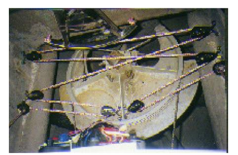
**CH** quadrant mounted down, lines connected forward of the rudder stock have to be crossed. (Bénéteau Oceanis 39).
