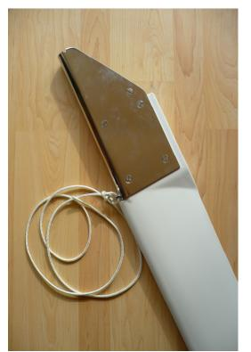
Power generated by the servo-pendulum is proportional to its wetted area and to the <u>square</u> of the speed of the boat. From this, we conclude that servo-pendulum area is <u>critical only at low</u> <u>speed</u>. At higher speeds, the pendulum generates considerably more power than needed to steer the boat.
