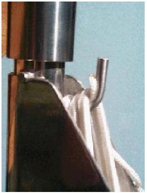
The easier way to connect the steering oar to its stock is first to hook the shock cord to the stock, then swing the steering oar in position over the stock until the two pins are snug into the notches.
