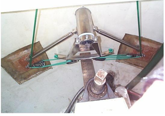
**CH** quadrant below axle, control lines led to blocks fastened on a short auxiliary tiller clamped on rudder stock (Pan Oceanic 43).
