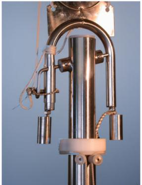
balance the weight of the connecting rod inside the windvane tower; the higher the tower, the more the counterweights have to be offset to the side to balance the added weight.
