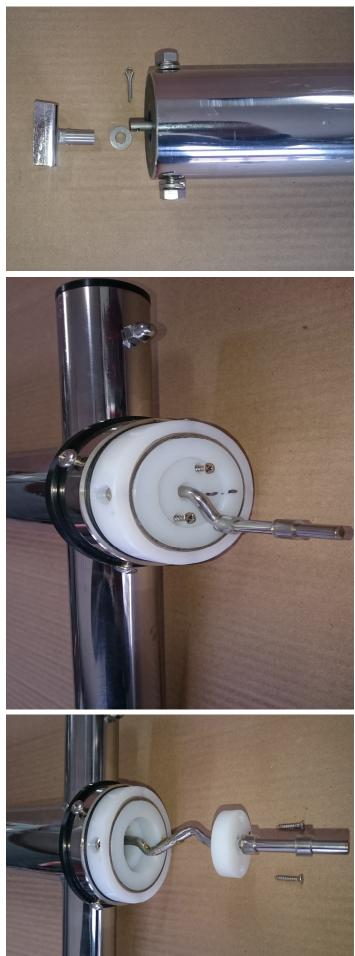
When re-assembling, the precise position of the co-axial control rod , both fore-and-aft and lateral, is critical to ensure that there is no friction between the control rod and the stock of the servo-pendulum.
