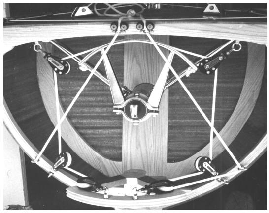
**CH** quadrant mounted in the "UP" position, lines connected to the rudder quadrant forward of the rudder stock. Jamming cleats placed close together (**Cape Horn** display model)
